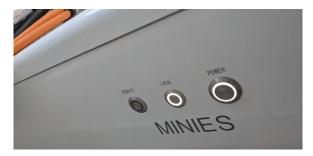
To switch the system into remote mode press and hold the remote button until the illumination on the local button goes out this generally takes 6 seconds, now when you release the remote button it should be illuminated as shown below.
