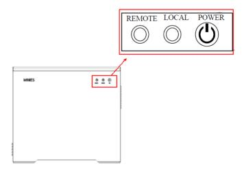
Two of the 3 buttons should have an illuminated halo one of which will be the Power button and then either Remote or Local will be illuminated, indicating which mode the battery system is in.
